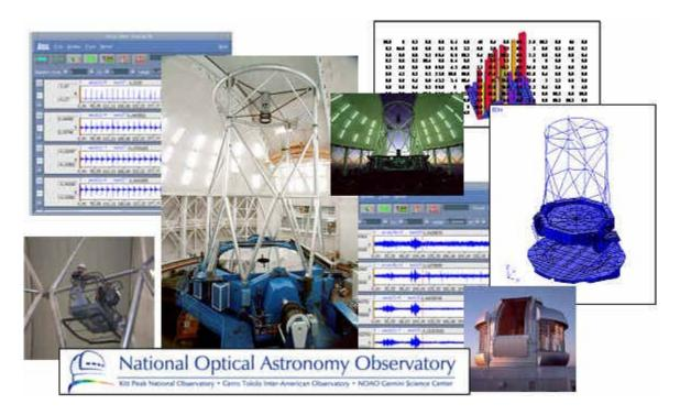
Traditional modal tests in conjunction with operating data helps to better understand the dynamic characteristics of large structures to determine the structure's response and modal participation of important modes
