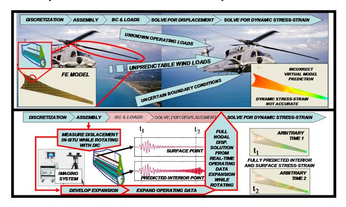
Conventional approaches for identification of structural response are limited by the ability to identify the force driving the system, identification of system configuration and identification of the actual system/component boundary conditions. Novel techniques have been utilized to approach the problem from a completely different perspective.
