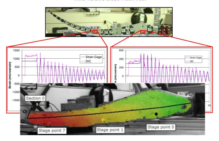
Digital Image Correlation results compare very well to traditional strain measurements as shown for a typical blade pluck test performed. The DIC has a big advantage in that full field strain results can be obtained.
