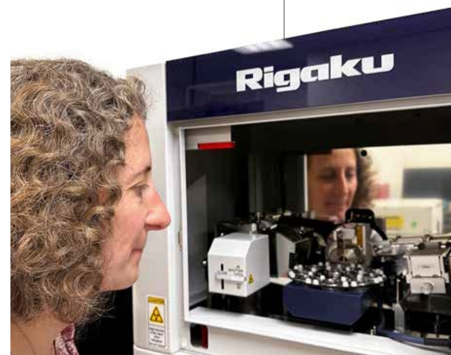
Assoc. Prof. Kate Swanger looks inside an X-ray diffractometer, which analyzes the structure of crystals.
