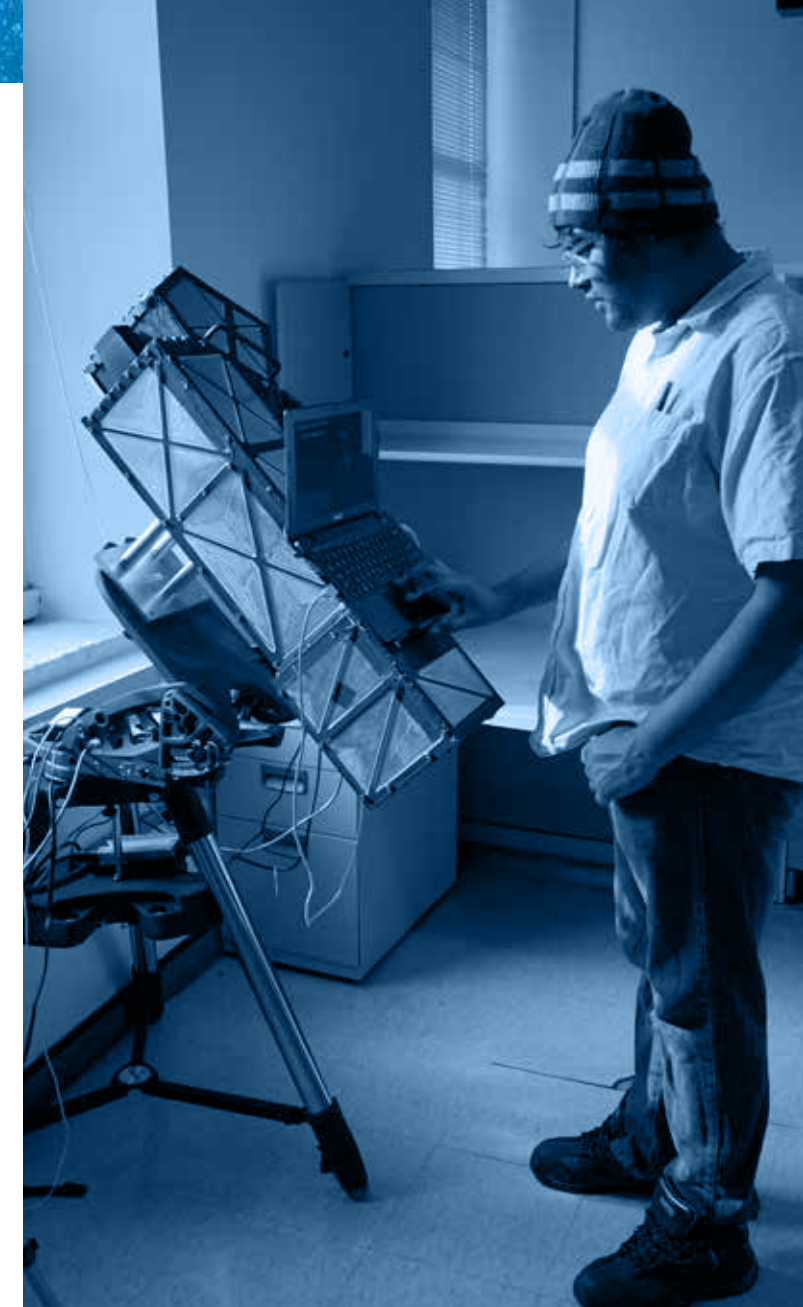
Sunip Mukherjee '23 studies visible light emissions from the ionosphere using a spectroscopic imager at LoCSST.
