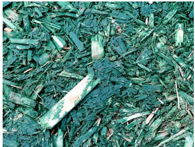
EWF dyed green and bonded together with chemical adhesive on a playground in Westford, MA.
