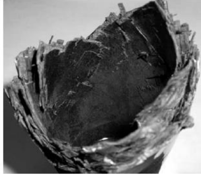
Figure 15. Low durability baseball bat that had barrel separation from a NBI. [21]
