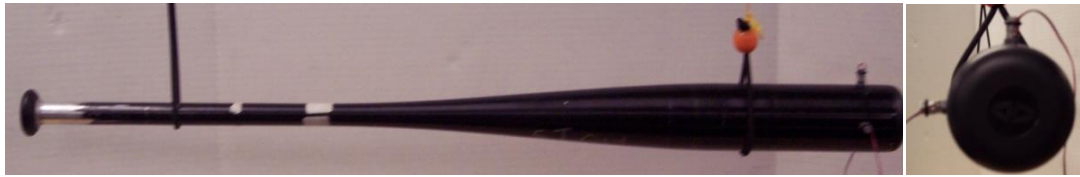
Figure 23. Simulated free-free impact modal test setup.
