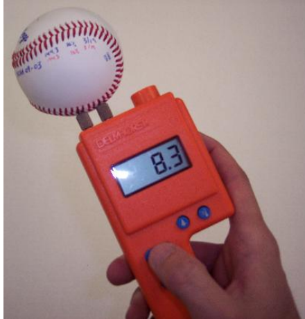
Figure 31. Measuring the moisture content of a baseball.
