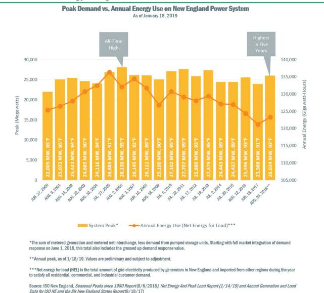
Fig. 3. Peak demand and annual energy use on New England Power System between years 2000-2018. Retrieved from https://www.iso-ne.com/about/key-stats/electricity-use/
