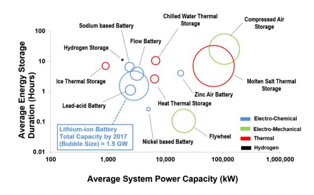
Fig. 5. Average characteristics of energy storage systems built worldwide between 1958 and 2017. Retrieved from https://www.nrel.gov/docs/fy190sti/71714.pdf
