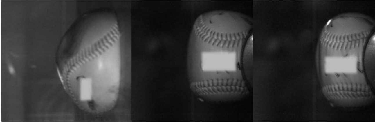
Figure 4: High-speed video frames of impact for Model A [Left: 26.8 m/s (60-mph) COR, Middle: 26.8 m/s (60-mph) CCOR, and Right: 40.2 m/s (90-mph) CCOR]
